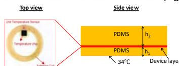
Fig. 4 The sensor components and the magnetic loop antenna for wireless power and data transmission are located between two soft layers of the elastomer poly(dimethylsiloxane) (PDMS) to ensure durability and to provide soft interfaces with excellent thermal coupling to the skin.
