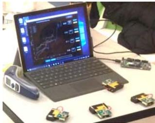
Fig. 3 The reader system includes a reader card, readers, and the logging software.
