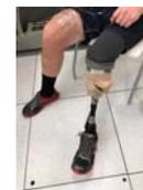
Fig. 7 Readers attached to exterior of prosthesis
